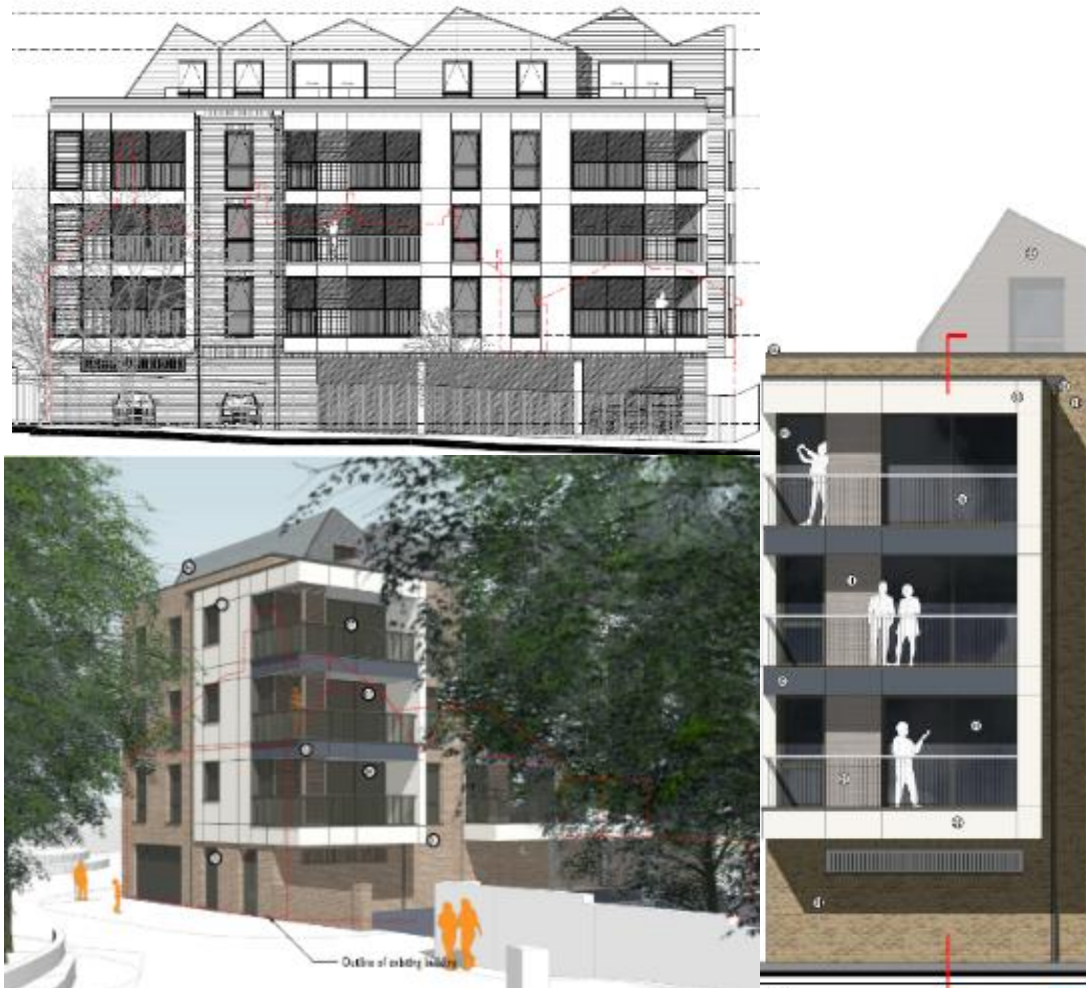
SOUTH ELEVATION, CORNER DETAIL, AND BALCONY DETAILING
